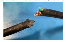
In a previous incident, also involving a profiling bed and a hybrid mattress pump, a member of staff sustained a fracture from a trip incident where the power cable had been incorrectly routed from a hybrid pump at the foot end of a bed to the wall socket at the head end along the floor around the outside of the bed.
