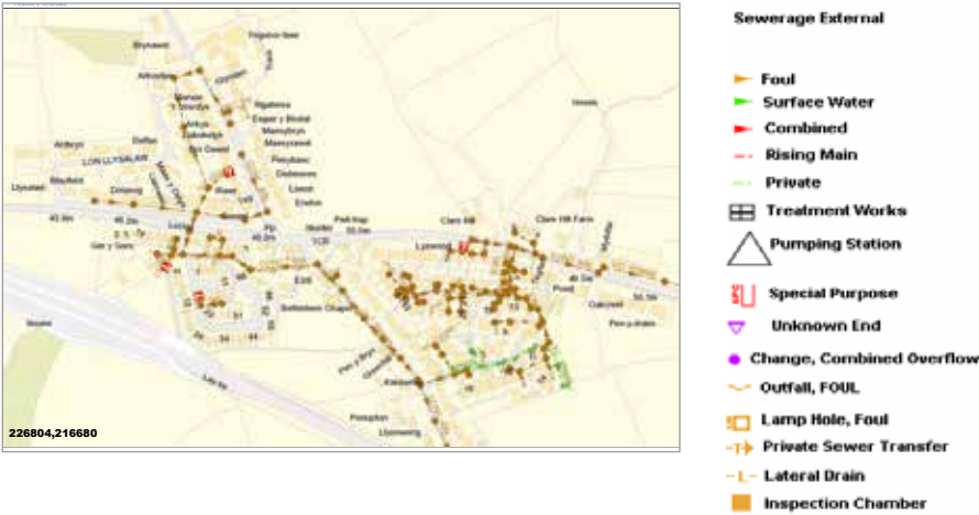
Fig. 2.1 - Existing sewerage infrastructure in Pwll-Trap
