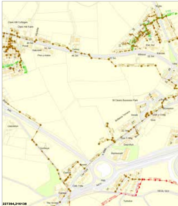
Fig. 2.1 - Existing sewerage infrastructure
